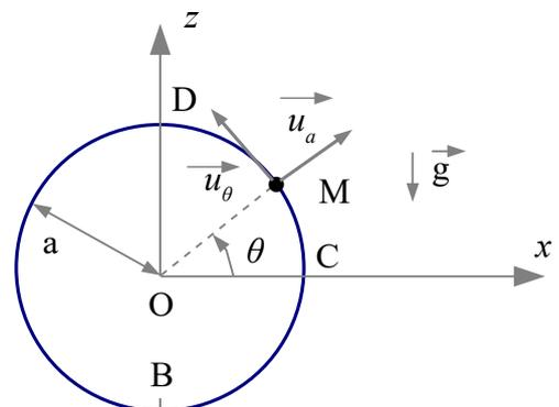
$$-am\dot{\theta}^2 = -mg \sin \theta - R \quad \text{soit} \quad R = am\dot{\theta}^2 - mg \sin \theta \quad \text{or} \quad V_M = a\dot{\theta} \quad \text{d'où} \quad R = m \frac{V_M^2}{a} - mg \sin \theta \quad \text{en}$$
